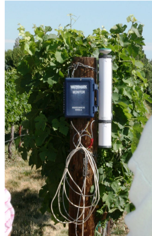
Monitoring soil moisture and ET are needed to determine when and how much to irrigate. Photo by Patty Skinkis
